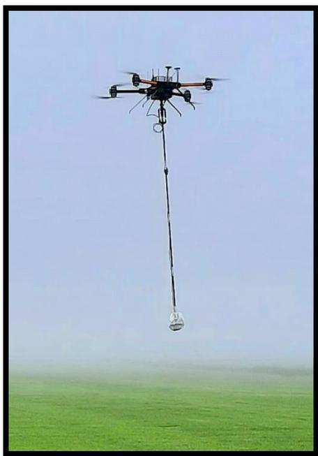
Surveys will cover 12.75 square kilometres at a 50m flight altitude using a 50m line spacing for a total of 285 survey line-kilometres.
